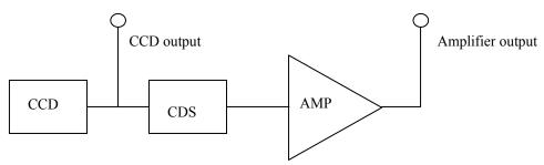
The output voltage is measured at the CCD output.
